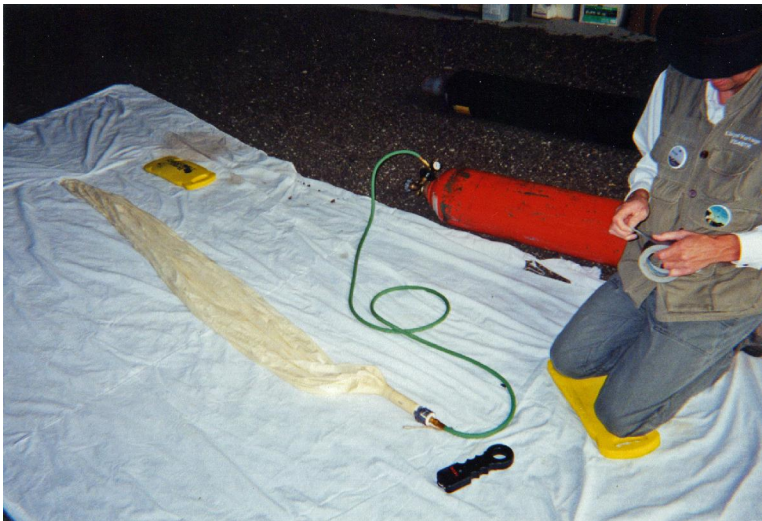
Launch Support Equipment – The author preparing to fill a balloon, using readily available equipment. None of the launch equipment is special order.
