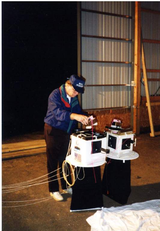
Bill All (N3KKM) – Preparing two modules in a near spacecraft for a very early morning launch. Each airframe costs less than $50. and is totally reusable.
