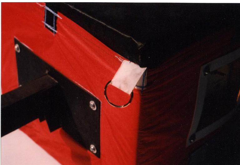
Dacron Link Loop - A four inch strip (of doubled over) Dacron is sewn into all eight corners of the abrasion jacket. One-inch split rings are slipped into the Dacron loops so that modules can quickly be linked together with link lines.
