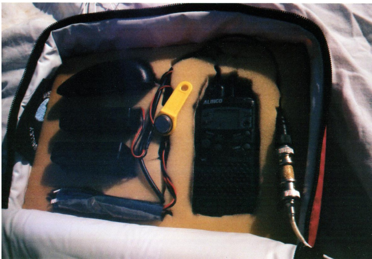
Interior of Lunch Bag Airframe -The interior of Jeff Melanson's (K7INN) lunch bag airframe. Inside, the GPS, TNC, HT, and a thermochron are cushioned with foam rubber.
