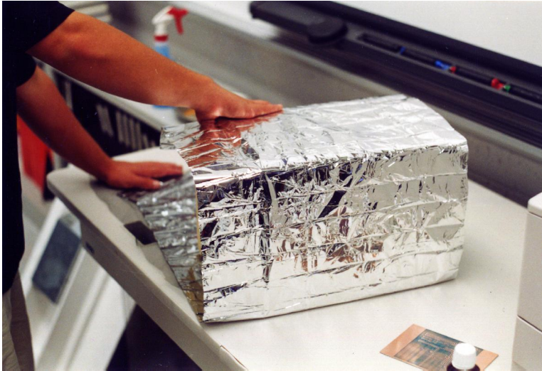
Wrapping airframe in MLI - Wrap the airframe in a strip of space blanket and scrim.
