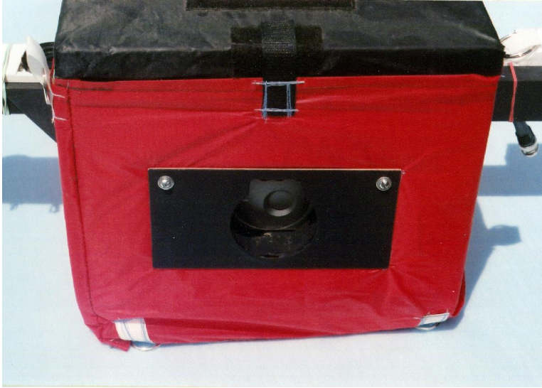
Velcro Closure - Centered at the top of each face of the abrasion jacket is a Velcro tab. It is used to secure the hatch to the airframe.
