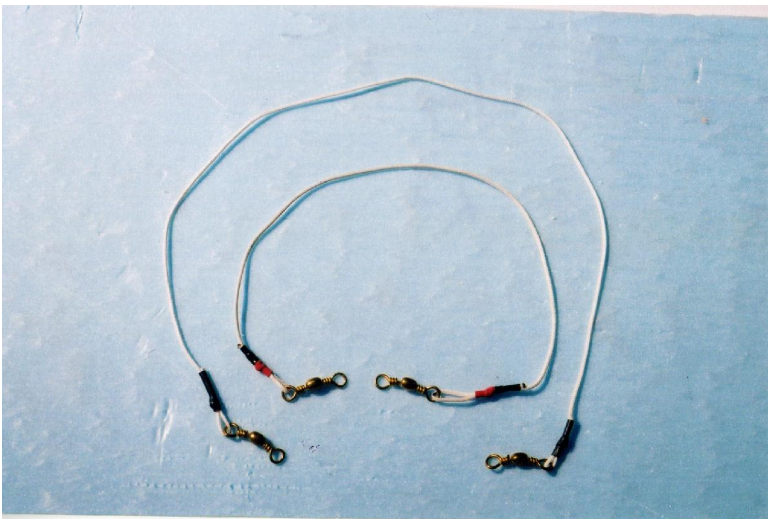
Two Link Lines - The colors of their heat shrink tubing indicates their lengths.
