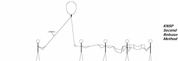
The first flight this method was used on, successfully launched the near spacecraft in higher winds that KNSP was accustomed to, however, one of the lanyards remained in front of the slow scan
