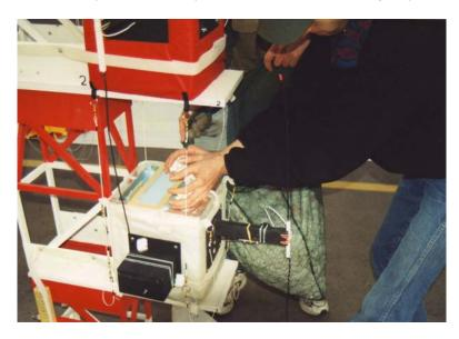
*Filling module with packing peanuts – Note the peanut bag*
