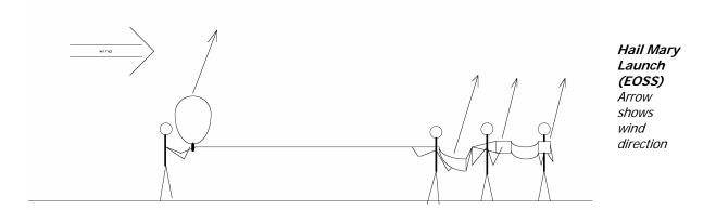
TVNSP has used this method to launch in high surface winds. The stack was released in the wind shadow of a building.
