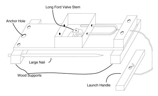
Simply place a long Ford tire valve stem in the 5/8 inch hole. Attach the pump to the stem and place the 2-liter pop bottle on the flat end. One or two washers may be placed under the valve stem to raise it thus pushing it farther into the bottle throat forming a better seal.
