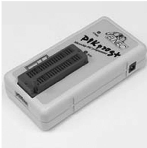
**Figure 5.16: PIC Prog Plus programmer**
