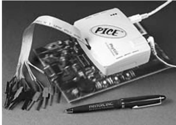
**Figure 5.23: PICE-MC in-circuit emulator**
