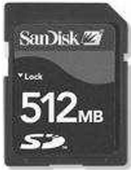
Figure 7.1: A typical SD card
