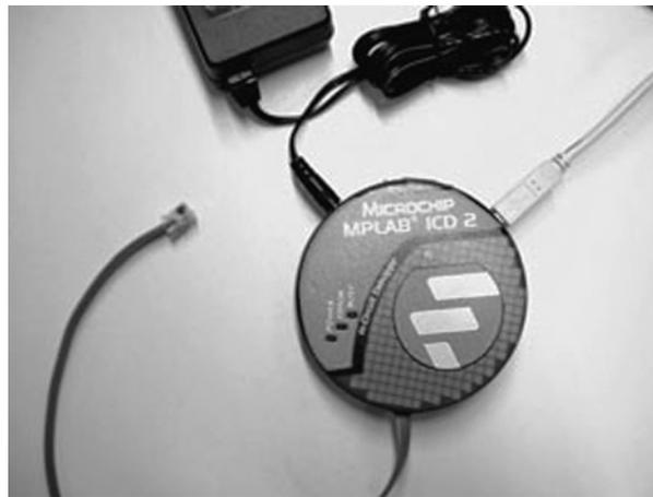
**Figure 5.17: ICD2 in-circuit debugger**
