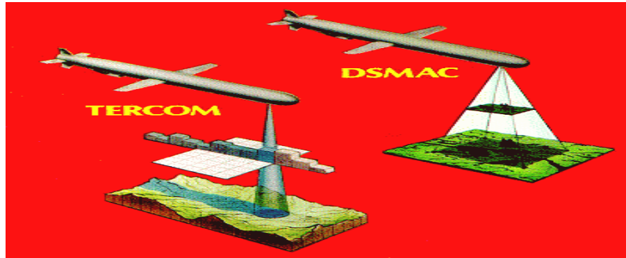
Terrain Contour & Digital Scene Matching Guidance (BGM-109 Tomahawk)
