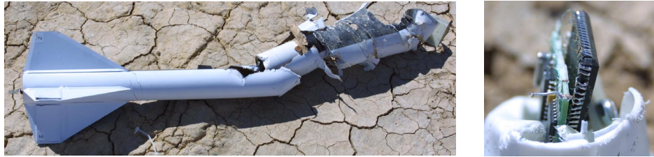
Photos of damage to Rocket 2, Payload B after recovery failure
